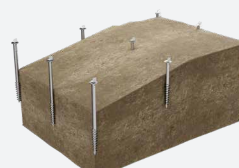
Step 1 Foundation screw installation
