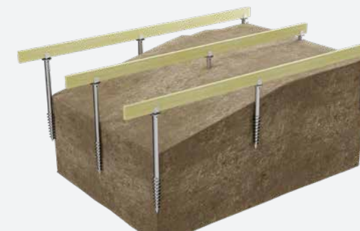
Step 2 Beams installation
